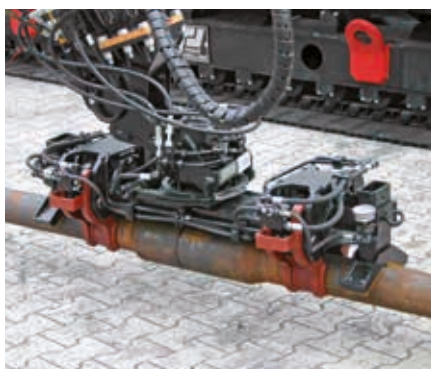
3D drill pipe gripper, rotatable and swivelling
