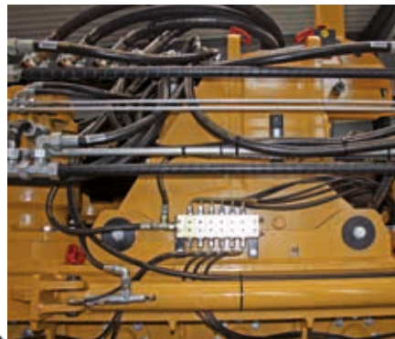
Automatic central lubrication unit
