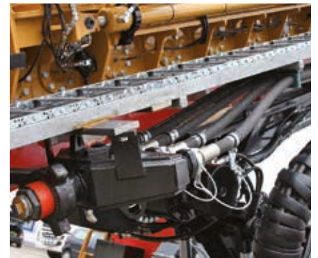
Mud supply, hydraulically lockable with by-pass
