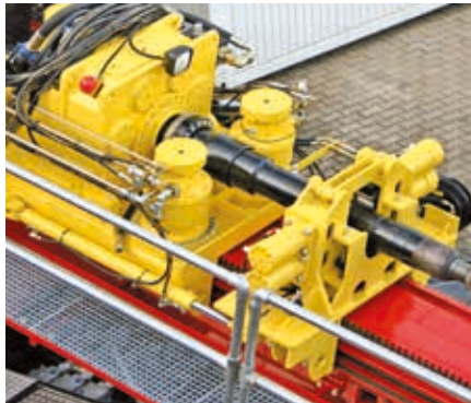
Breakout system at the power rotary head
