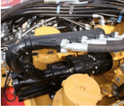
Mud-swivel Western type with manifold
