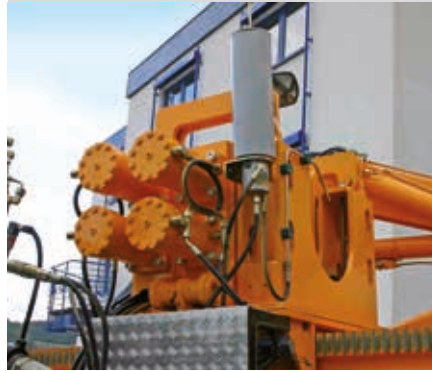
Automatic drill pipe lubrication
