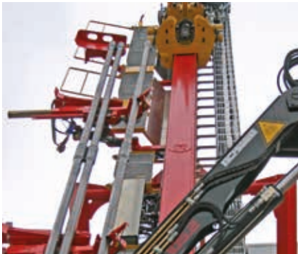
Drill pipe supply for 5 drill rods
