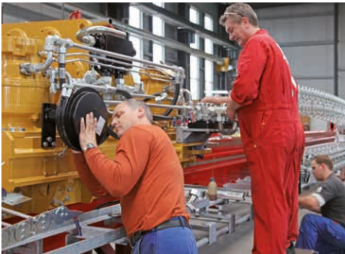
Assembly work on the power rotary head
