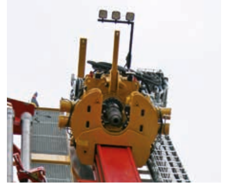
Camera and lights for power rotary head and breakout unit
