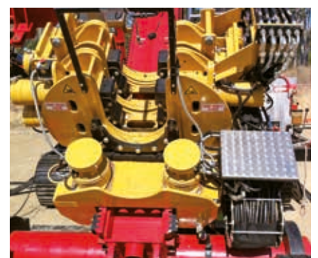
Breakout system with easily replaceable and self-centering clamping jaws
