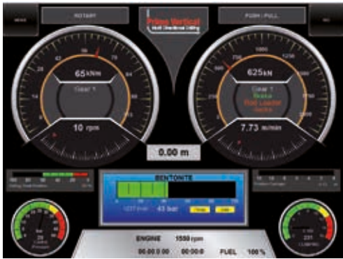
Drill data log system for recording of drilling parameter
